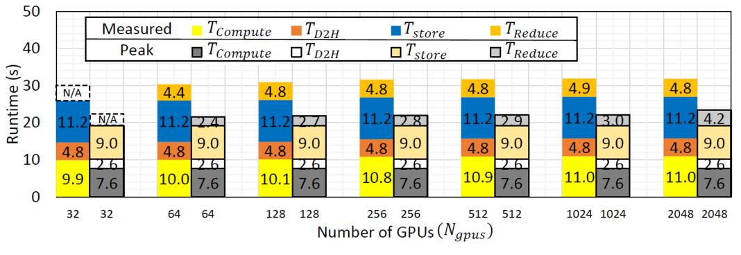
Weak scaling for  $2048^2 \times N_p \rightarrow 4096^3$ .  $N_p = 16^* N_{gpu}$
